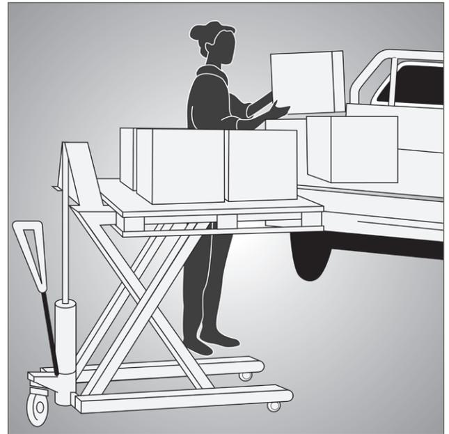
Figure 35 – Scissor pallet jack open pallet
