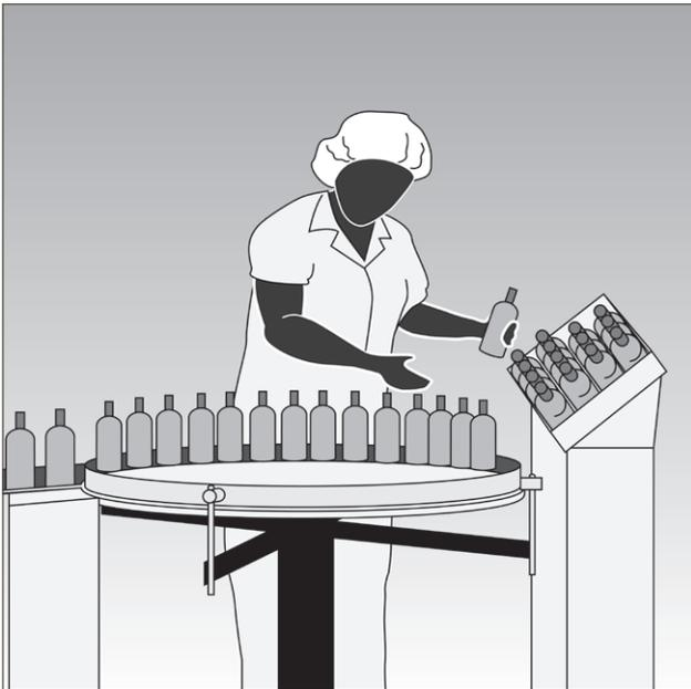
Figure 39 – Turntable for buffering products
